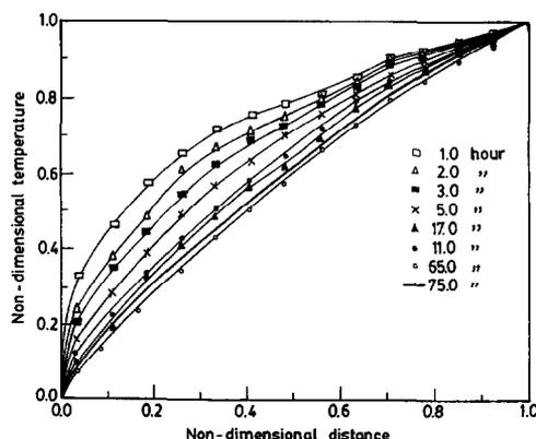
Fig. 3. Variation of temperature with time at specific distances (cm).
