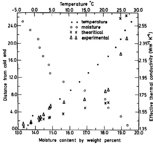
Fig. 4. Variation of effective thermal conductivity (ETC) with moisture content and distribution of steady-state temperature and moisture with axial distance from cold end (cm).
