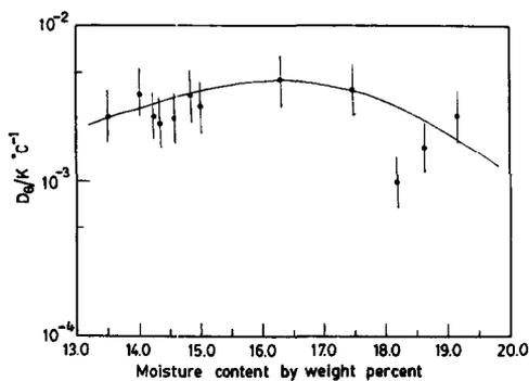
Fig. 5. Variation of the ratio of thermal and moisture diffusion coefficients with moisture content.
