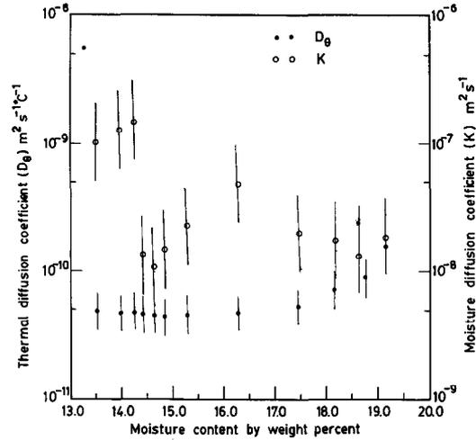
Fig. 6. Variation of thermal and moisture diffusion coefficients with moisture content.
